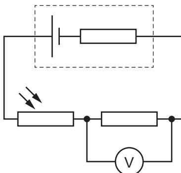
The voltmeter reading increases.
