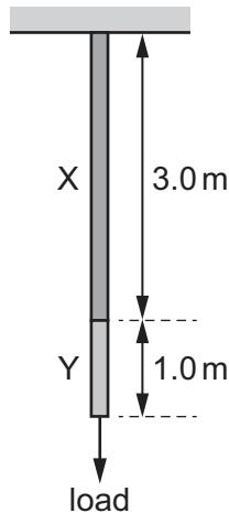
A load hung from the wire causes metal X to extend by 1.5 mm and metal Y to extend by 1.0 mm.
