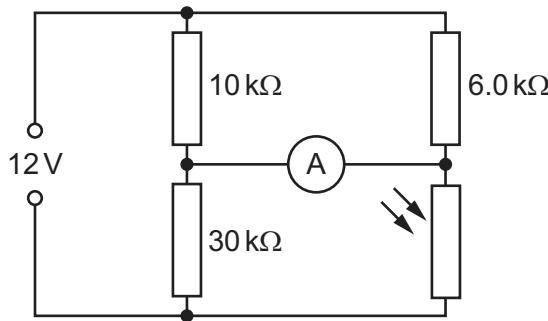
The ammeter reads zero current.
