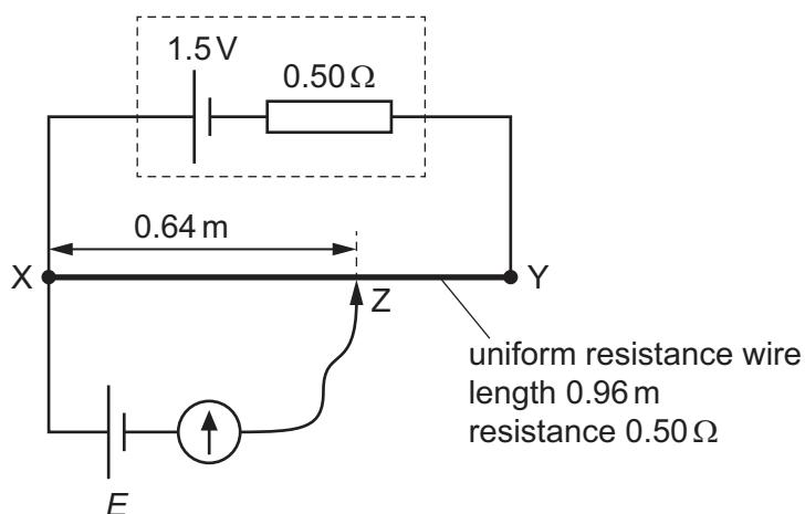
The resistance wire XY has a length of 0.96 m and a resistance of 0.50  $\Omega$ .
